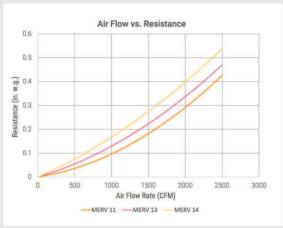
\*Technical data is based on a 24" x 24" x 30" 8 pocket filter.
