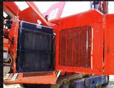
Drilling Rig Air Intake
