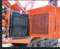
Drilling Rig Air Intake
